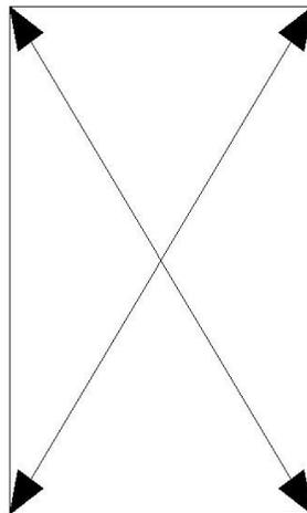
2. Using a tape measure, check the rough opening. Measure diagonally across the opening. Diagonal measurements need to be equal within  $\frac{1}{4}$ ".
